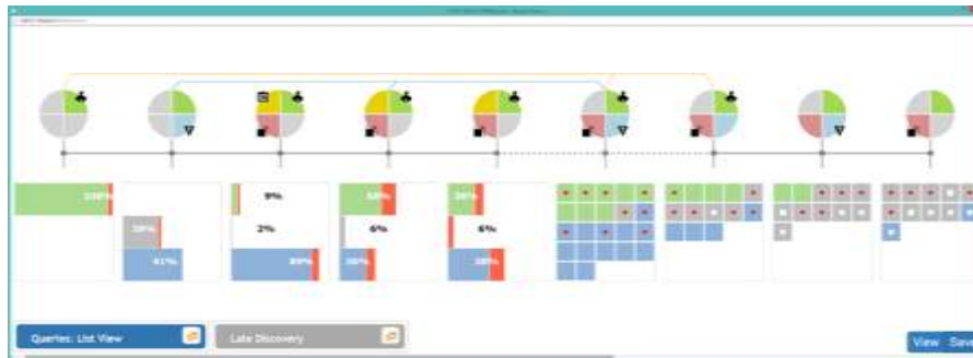
Figure 12: An example of glyph-based visualization of the queries selected in Figure 11. The search queries are shown above the central line, and the search results are shown beneath the central line. Each search query may feature four criteria of (in clockwise direction): keyword, type, size, and date. An icon appears when this criterion is new or has been changed. The search results are shown in two forms: summary statistics are shown when research results consist of more than 25 files and macro-glyph otherwise. For search results, green represents newly found files, grey represent files common to the current and previous queries, blue represents files appeared only in the previous query, and red represents the selected files. The background colour of the 'Late Discovery' dialog is grey as there is currently no newly discovered file. Adopted from [Kha15].
